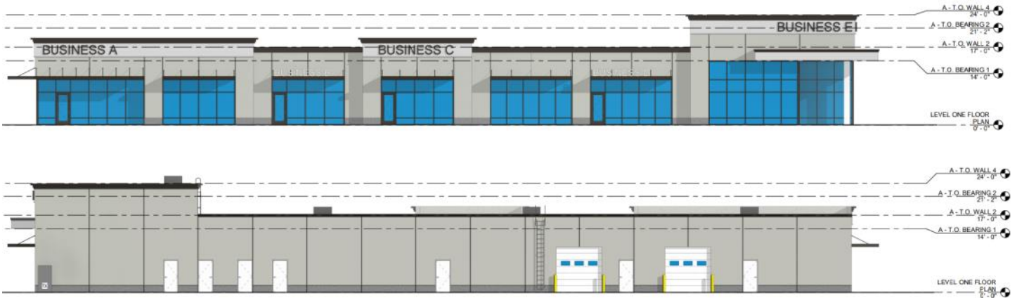
4 BUILDING A - EAST ELEVATION 1/8" = 1'-0"
